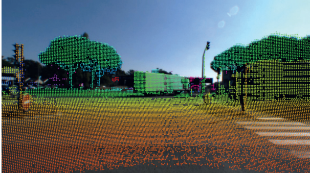
Calibrated data. Lidar data projected on camera image.
