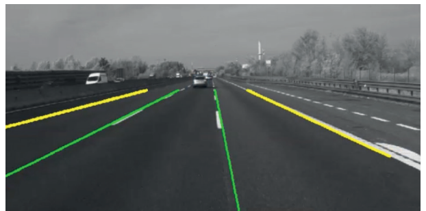
Line detection using image processing.
