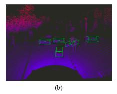
**Figure 9.** Object detection by DCNN: (a) camera image for illustration and (b) result of lidar DCNN detection.
