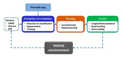
Figure 1. Modular architecture of automated driving system.
