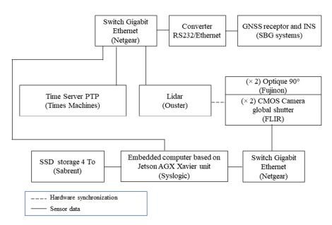
Figure 3. Data and synchronization communication scheme.
