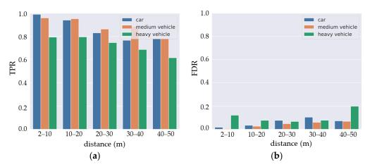
Figure 11. DCNN detection results: (a) true positive rate and (b) false discovery rate.
