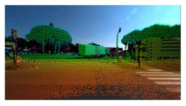
Figure 6. Lidar point cloud projected onto camera images.
