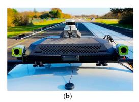
**Figure 2.** (a) Perception and localization system installed on an experimental vehicle; (b) zoom of the PLS.
