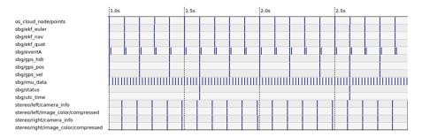
Figure 5. Timeline of data acquisition from the perception and localization platform's sensors.
