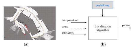
**Figure 13.** Lidar-based localization algorithm: (a) map building process and (b) localization operating schemes.
